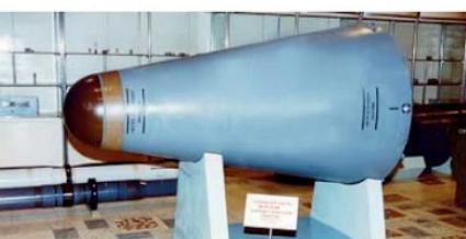
1963 deployed Russian megaton SLBM warhead, length 230 cm, diameter 130.4 cm. Mass 1144 kg.
